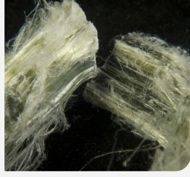
Asbestos easily breaks up into fibers
